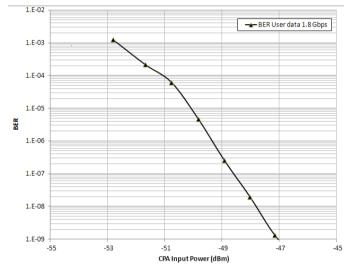
Figure 8. BER of LCT versus LCT CPA input power
