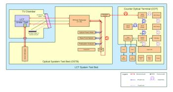
Figure 6. The optical system tesbed for testing the Alphsat LCT (not all units of the generic OSTB shown are used)
