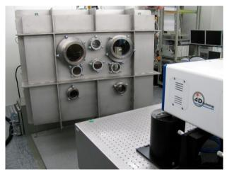
Figure 5. Thermal vacuum chamber for LCT performance verification with several optical windows for LCT access. The bigger windows allow access to the LCT CPA aperture to perform communication and wave front error measurements, while smaller windows allow acces to the LCT pointing reference cube for pointing verification.
