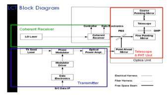
Figure 1. Tesat LCT block diagram.
