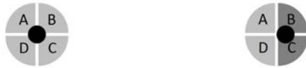
Figure 10: Spot position on the 4QD. Left: spot in the center - no PID-controller adjustment of FSM needed. Right: spot outside center - PID-controller adjustment of FSM needed [7]
