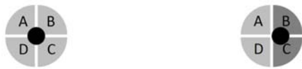
Figure 10: Spot position on the 4QD. Left: spot in the center - no PID-controller adjustment of FSM needed. Right: spot outside center - PID-controller adjustment of FSM needed [7]
