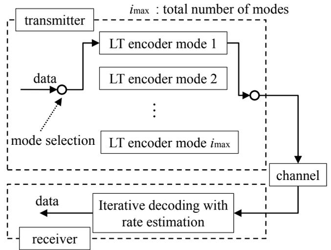
Fig. 3 Block diagram of multi-rate LT codes transmission.
