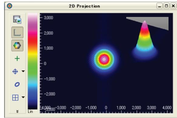
Fig. 4. The beam quality of testbed laser output at energy of 20 mJ, 15 ns.
