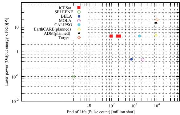
Fig. 2. Power and end of life of laser transmitter for current and planned space borne LIDAR system.
