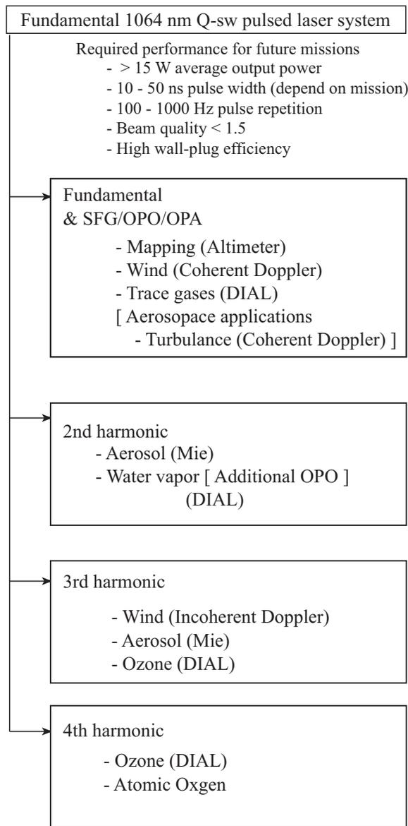
Fig. 1. Expected missions with high-end performance LIDAR.
