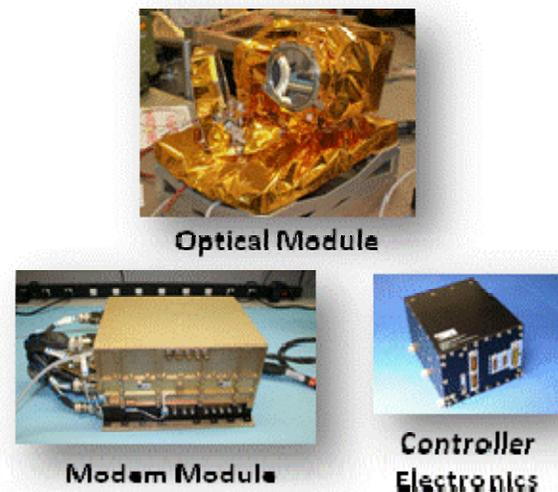
Figure 1. The Lunar Lasercom Space Terminal (LLST)
