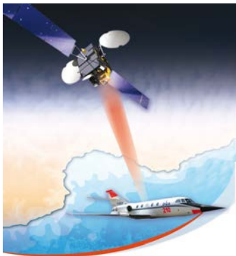
Figure 2: LOLA bi-directional optical data link between an aircraft and Artemis GEO satellite
